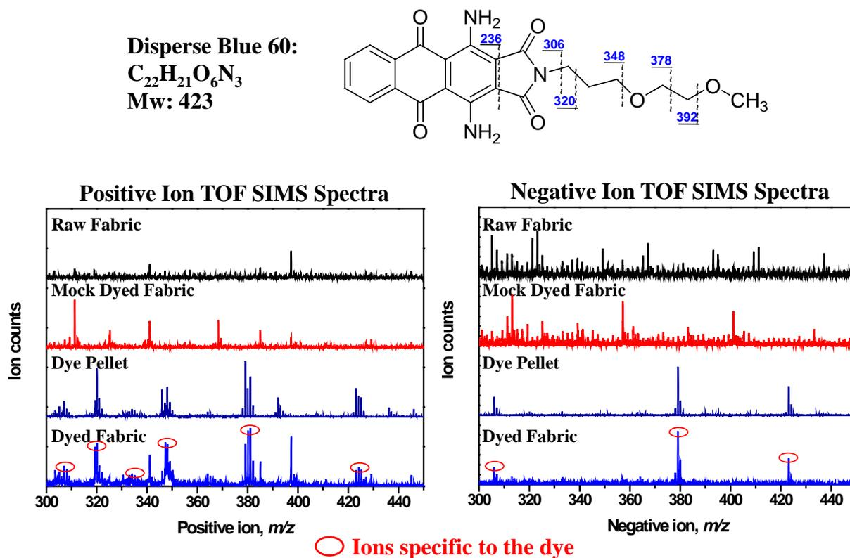
Figure 2. The molecular structure of Disperse Blue 60 and the positive and negative TOF SIMS secondary ion spectra of the raw fiber, mock dyed fiber, dye pellet and the dyed fabric (7% owf) are presented. The masses of possible stable molecular fragments are shown in blue on the molecular structure. Secondary ion peaks attributable to Disperse Blue 60 dye (see red circles above) are present only in dyed fabric, not in raw fiber or mock dyed fiber.
