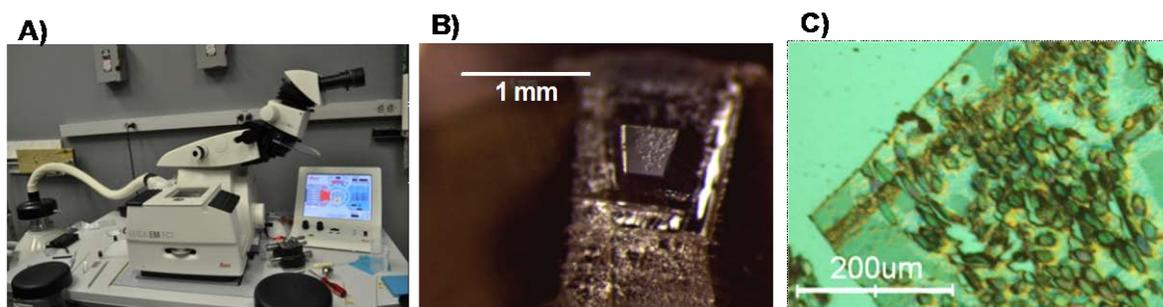
Figure 1. A) The Leica Ultracut EM UC 7 used in the project, B) a light micrograph of a representative block face with fibers embedded and C) a Nomarski filtered optical micrograph of a representative embedded, cryomicrotomed Disperse Blue 60 dyed polyester fiber cross section.
