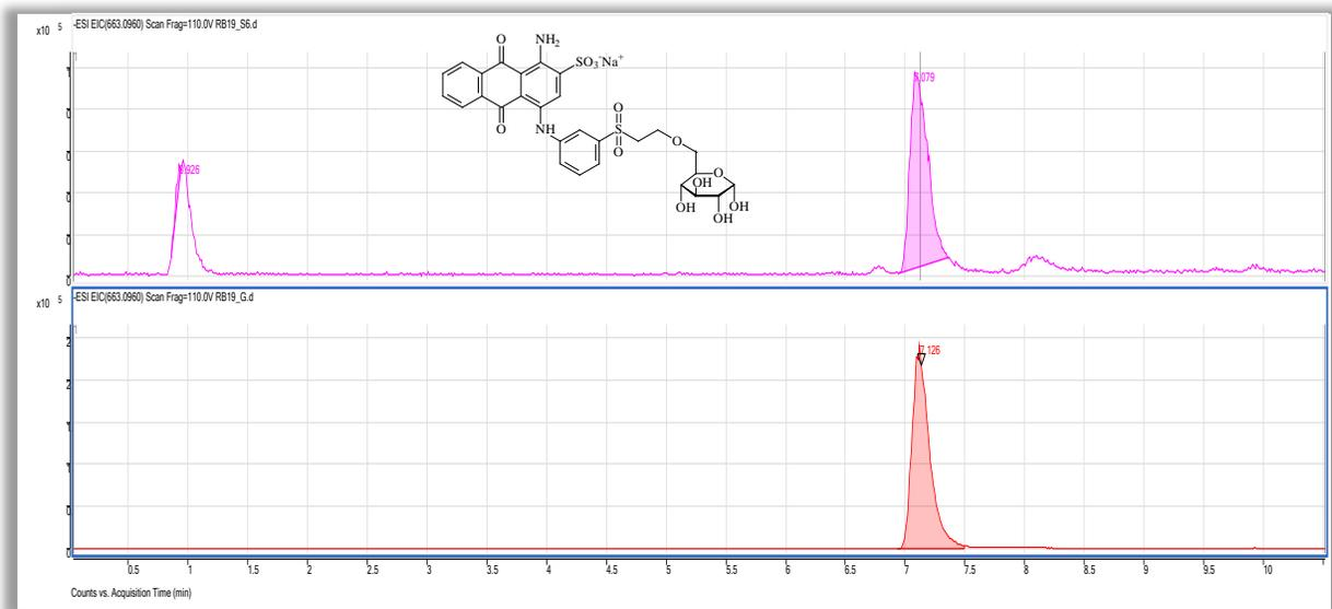
Figure 21. Comparison of diode array chromatograms obtained at 660 nm for synthesized Reactive Blue 19 with glucose (Top) and Reactive Blue 19 extracted from cotton sample (Bottom).
