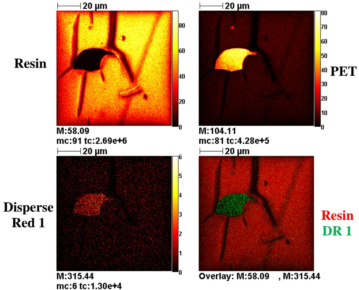
Figure 11. TOF SIMS images ( $100 \mu\text{m} \times 100 \mu\text{m}$ ) of a 5% owf Disperse Red 1 dyed polyester (PET) fiber cross section showing the spatial distribution of Resin, PET, the molecular ion of Disperse Red 1 and overlaid image of resin (in red) and the Disperse Red 1 molecular ion (in green). The images are reconstructed from 200 frames of  $256 \times 256$  pixels, 1 shot/pixel  $\text{Bi}_3^+$  data acquisition.
