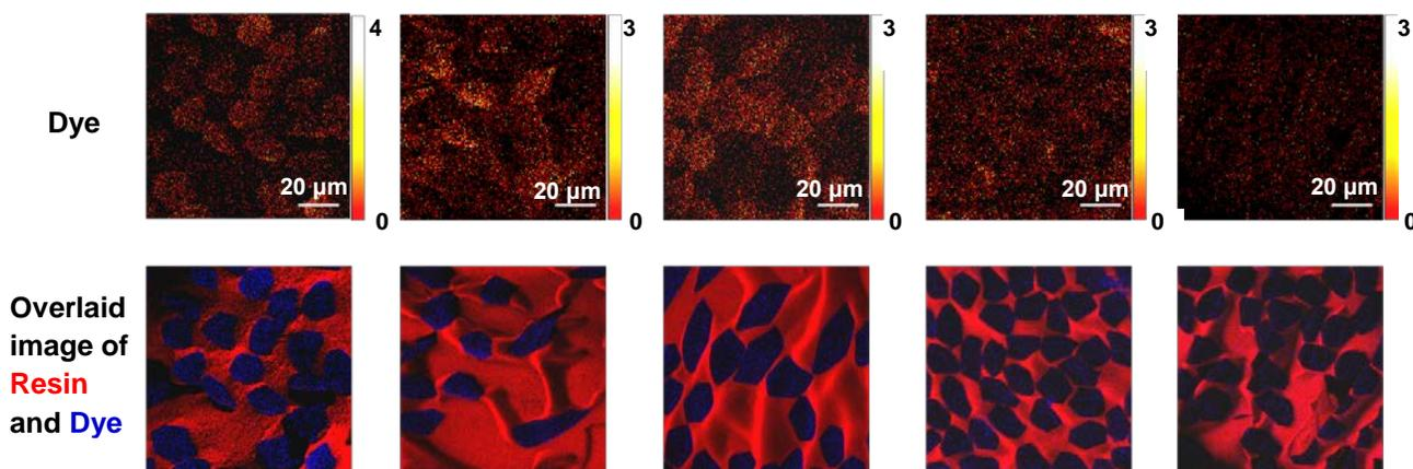
Figure 6. The top row of images are TOF SIMS images of the 379 molecular ion of Disperse Blue 60 for the dye loading given. The lower row of images has the dye (encoded in blue) overlaid onto the TOF SIMS secondary ion image of the embedding resin.
