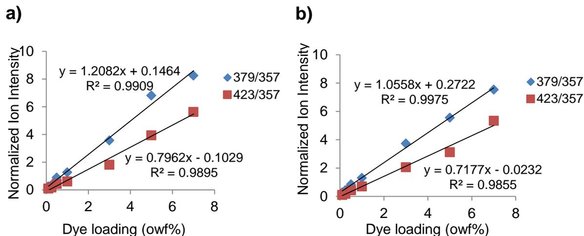
Figure 3. Normalized Disperse Blue 60 molecular ion intensities at  $m/z$  379 and  $m/z$  423 dye components versus dye loading obtained from fabric surfaces is presented. (a) The first set of Disperse Blue 60 dyed fabrics analyzed. (b) The second set of Disperse Blue 60 dyed fabrics analyzed.
