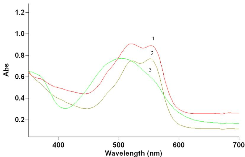
Figure 20. UV-Vis spectra for Reactive Red 141 with different digestion method at 45°C (1 – NaOH followed by enzyme treatment; 2 – enzyme treatment; 3 – NaOH treatment).
