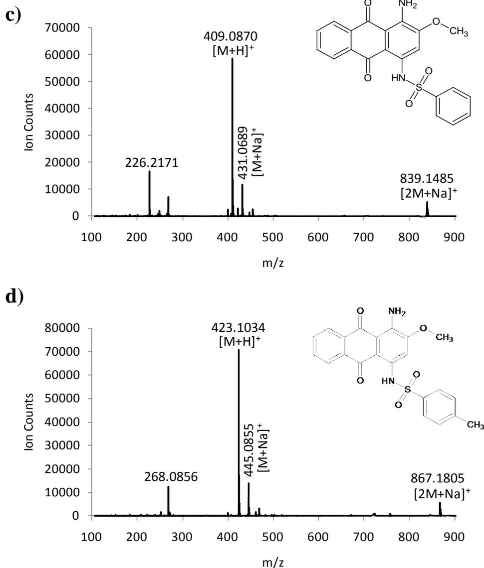
Figure 17. (a) Mass spectrum corresponding to peak at 7.62 min in diode array chromatogram of UK 04. (b) Mass spectrum corresponding to peak at 8.86 min in diode array chromatogram of UK 04. (c) Mass spectrum corresponding to peak at 7.63 min in diode array chromatogram of UK 08. (d) Mass spectrum corresponding to peak at 8.87 min in diode array chromatogram of UK 08.
