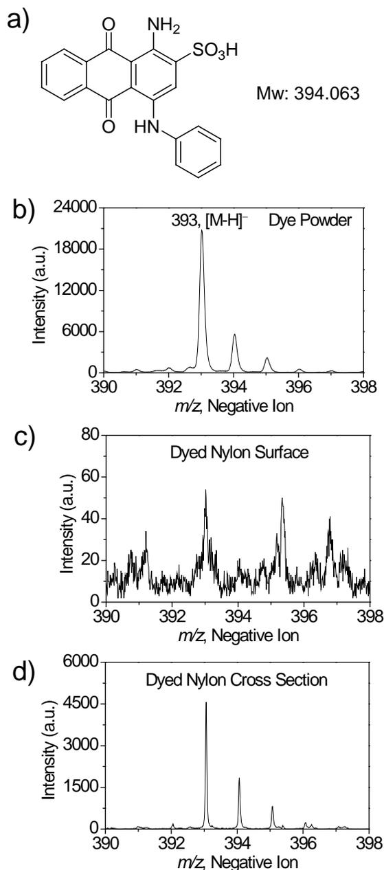
Figure 7. (a) Chemical structure and molecular weight of Acid Blue 25. Negative ion TOF SIMS spectra showing the molecular ion of Acid Blue 25 obtained from (b) dye powder, (c) 1% on-weight-of-fabric (owf) dyed nylon surface, and (d) 1% owf dyed nylon cross sections.
