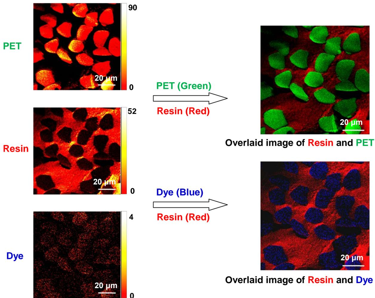
Figure 5. TOF SIMS secondary ion images of Resin (Red), PET (Green) and Disperse Blue 60 dye (Blue) are color encoded and overlaid to produce the images in the right column. The signal from Disperse Blue 60 clearly overlays with the PET.
