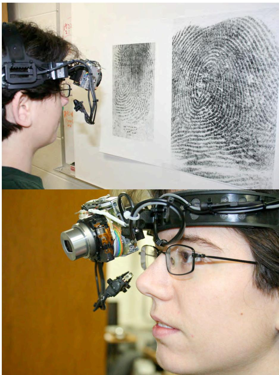
Figure 2. High Definition Eye camera that allows high-resolution movie capture during actual latent print examinations.
