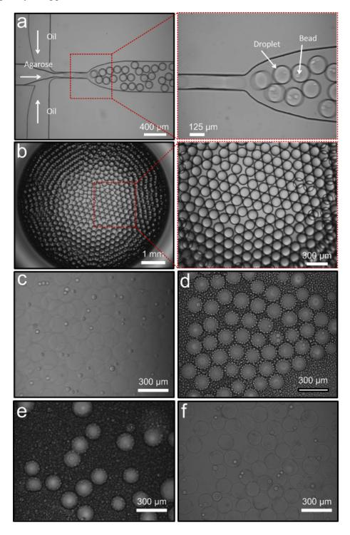
Figure 4. Agarose microdroplet generation and manipulation. (a) Microdroplet generation based on a flow-focusing structure of a PDMS/glass microfluidic device. Primer-functionalized beads and the desired number of cells (or
