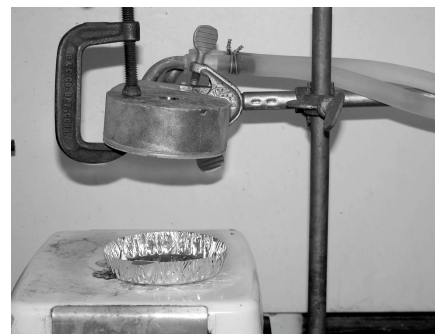
Figure 3: Fuming chamber with temperature control
