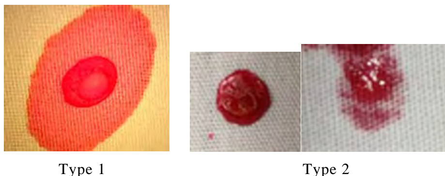
Figure III.2. Synthetic blood types 1 (SB1) and 2 (SB2) on textiles after being allowed to wick into the fabric and drying overnight.
