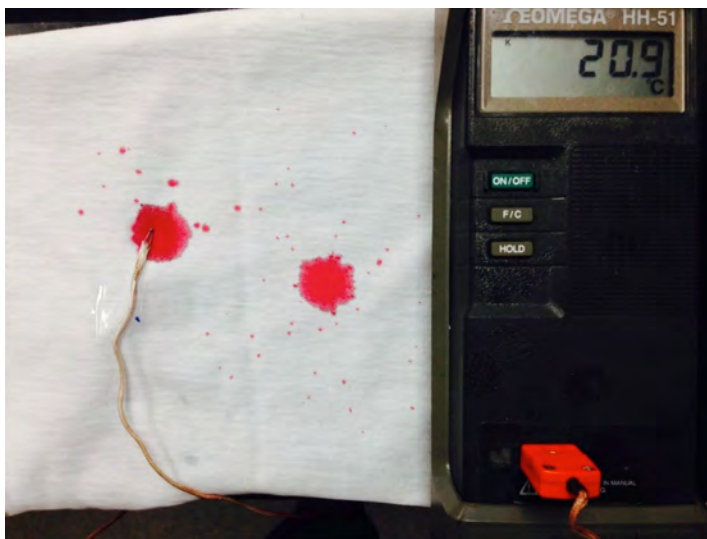
Figure II.1. Blood temperature measurement at impact after heating it to 37°C and dripping it 0.3 m onto the thermocouple and fabric.
