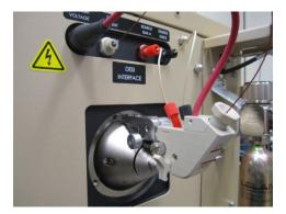
**Figure 3-1b.** Stock ionization assembly that allows both ESI (solution-based analytes) and DESI (surface-based analytes)
