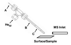
**Figure 3-3.** Depiction of the home-built LTP source. A discharge is produced between a (A) grounded electrode and (C) high voltage outer electrode, with a (B) quartz glass capillary serving as the dielectric barrier needed and ionization probe. The excited gas species produced can desorb/ionize surface-bound samples for MS analysis.
