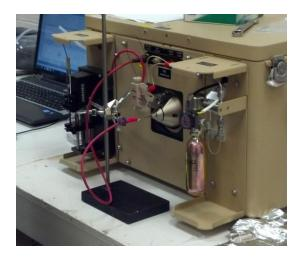
**Figure 3-4.** Depiction of paper spray ionization directly from a paper triangle containing analyte. By application of appropriate solvent and high voltage, deposited or swabbed analytes on the paper can be directly ionized/detected with the Flir Systems AI-MS.
