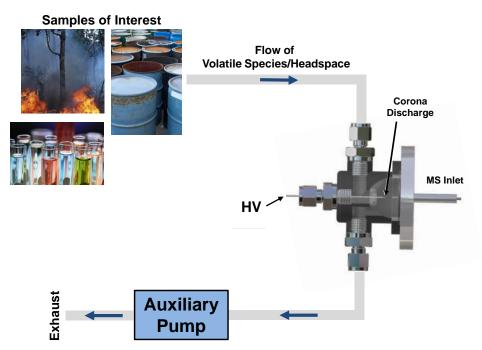
**Figure 2-2.** Basic design and usage of an APCI source to sample volatile chemical signatures from ambient air. An auxiliary pump continually draws fresh sample vapor through chemically-resistant PFA tubing into the corona discharge region. Resulting ions enter the MS inlet while the pump evacuates used sample through an exhaust port.
