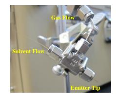
**Figure 3-2c.** Photo of the home-built DESI source, composed of a Swagelok tee assembly and fused silica capillaries for solvent flow and nebulizing gas.
