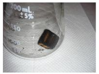
**Figure 3-26.** Post-burn wood block visibly charred and cracked after ignition with Coleman Fuel. Generated headspace can then be analyzed directly via APCI-MS
