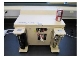
**Figure 3-1a.** Photo of Flir Griffin AI-MS instrument, with aluminum can in place for scale.
