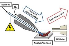
**Figure 1-1.** Schematic of the experimental setup for DESI-MS, allowing chemical analysis of untreated surfaces.
