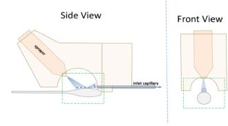
**Figure 3-2a.** Depiction of swab analysis using DESI. Charged droplets impinge upon the swab surface, desorbing/ionizing analytes present and projecting them toward the MS capillary inlet for mass analysis. Courtesy of Flir Mass Spectrometry.
