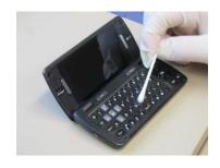
**Figure 3-19.** Depiction of using a transfer swab to probe the keyboard of a cellular phone for residues found in latent fingerprints.
