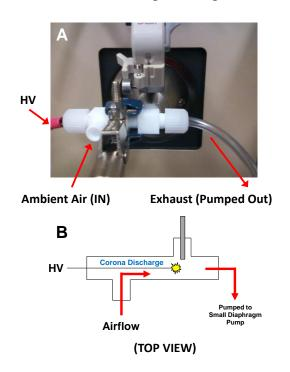
**Figure 3-25.** (A) Lightweight teflon APCI source attached to the Flir AI-MS 1.2 by simply lifting the DESI/ESI source in the maintenance position and sliding the source over the MS inlet capillary. (B) Top view schematic showing the interworking of the APCI source. The discharge needle is parallel to the flow of sample gas and perpendicular to the inlet capillary.
