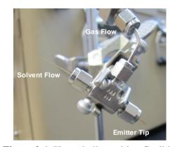
**Figure 2-1.** Home-built, position-flexible DESI source. A Swagelok tee assembly houses fused silica capillaries for solvent flow and nebulizing gas.
