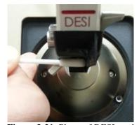
**Figure 3-21.** Photo of DESI swab analysis utilizing a swab positioning guide from Flir Mass Spectrometry.
