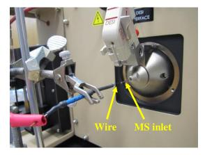
**Figure 3-22.** Simplified corona discharge APCI. High voltage is applied to a thin wire under resistivity. Gas analytes present between the wire and MS inlet are ionized and detected.
