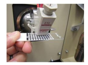
**Figure 3-2b.** Photo depicting direct analysis of a Teflon-coated glass microscope slide. Upon placement in the DESI spray, surface-bound analytes are instantaneously ionized and detected with minimal carryover
