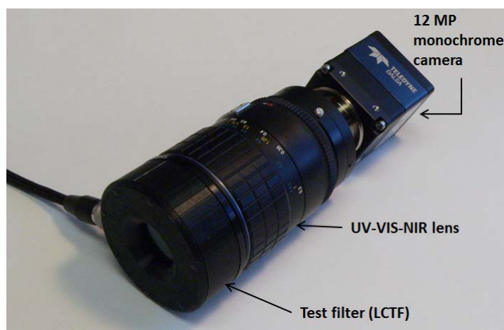
Figure 16. LCTF mounted to the UV-VIS-NIR lens and 12 MP camera
