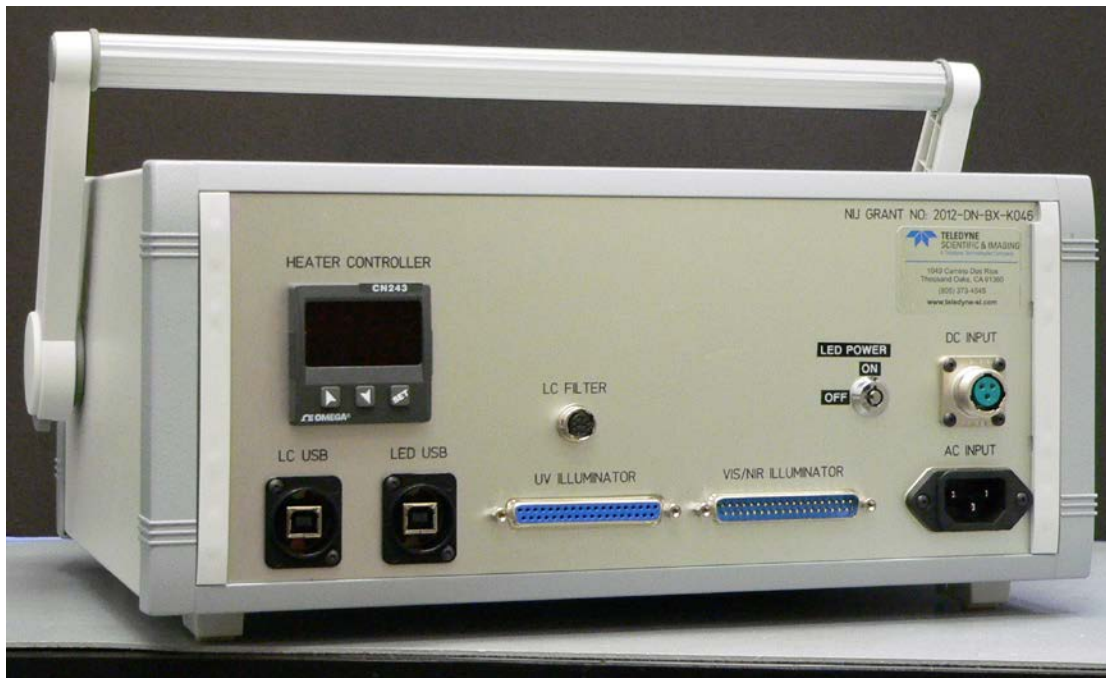
Figure 14. Controller electronics enclosure (back panel)
