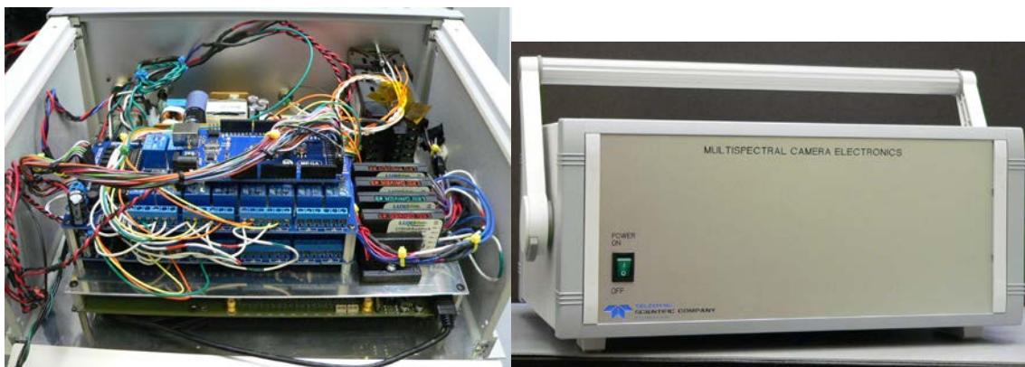
Figure 15. Integrated semi-custom electronics (inside and the front panel)
