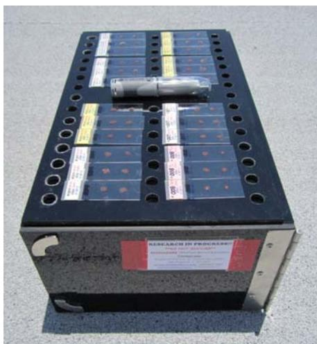
**Figure 7:** Black, opaque acrylic box for environmental damage to human bloodstains. Blocks UV light transmission, but ventilation holes allow exposure to heat and humidity. An internal tray that holds the samples is shown here (top) prior to being inserted into the box.
