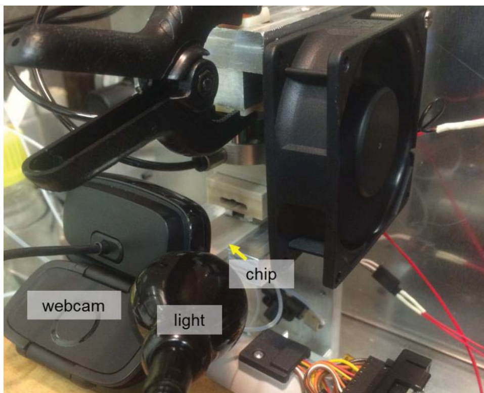
Figure 3-66. Cavity viewing setup
