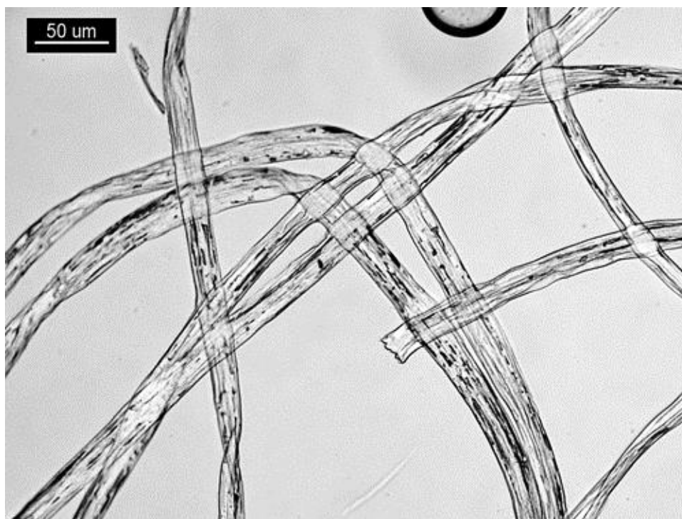
Figure 12. Plane polarized light image of A3 fibers after 24 weeks of freshwater submersion showing rectangular, elongated inclusions.
