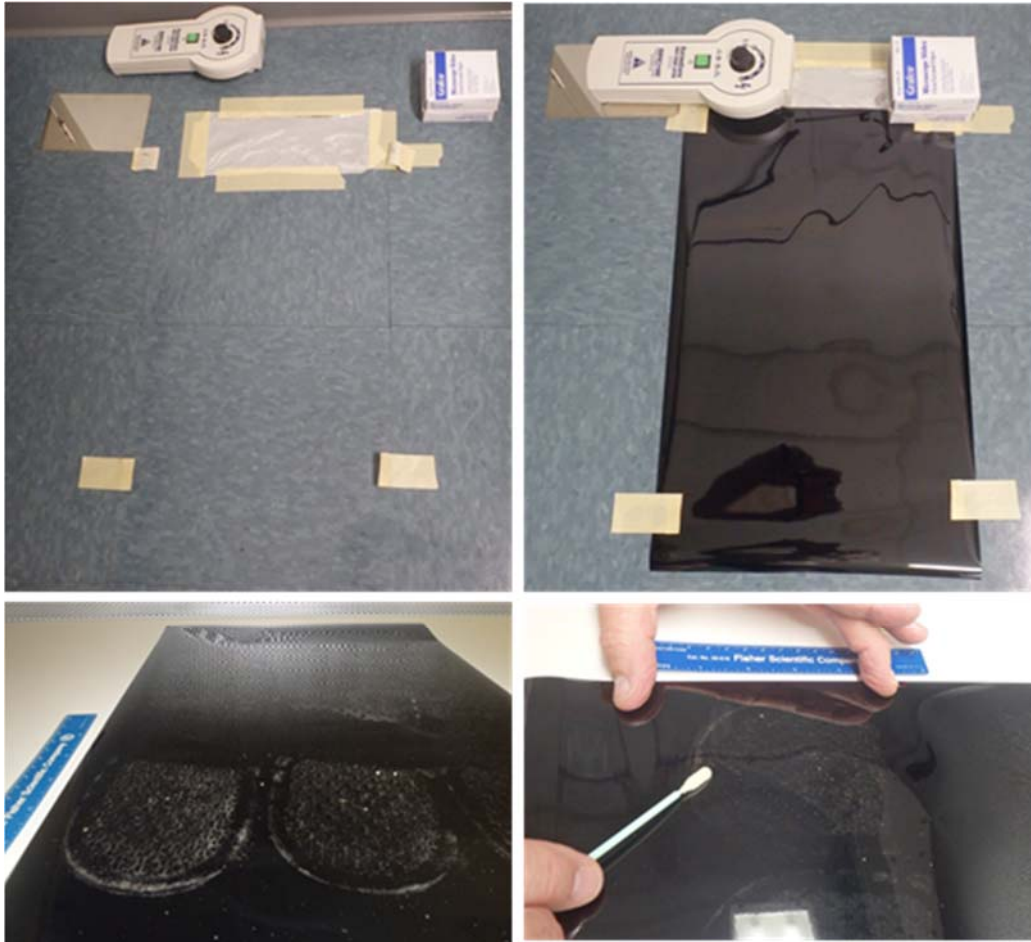
Figure 10. Removal of moderately held particles using an electrostatic lifter.
