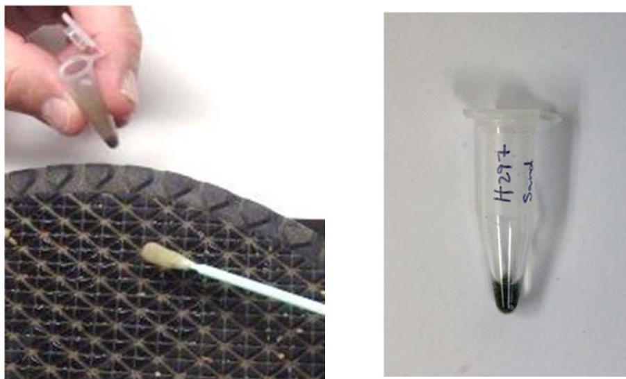
Figure 11. Removal of the most tightly held particles by direct swabbing of contact surfaces of the sole.
