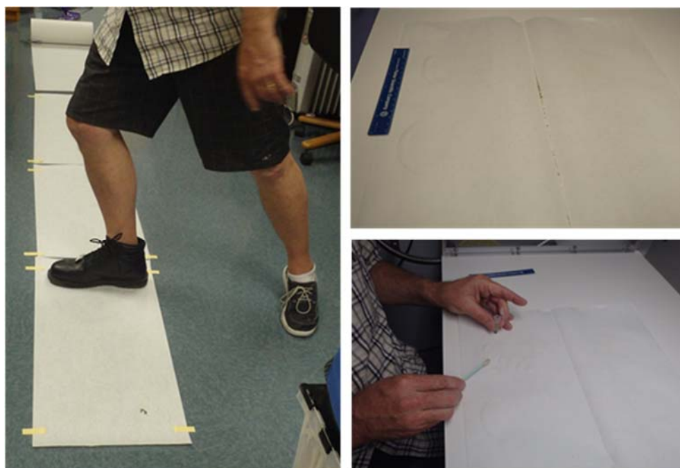
Figure 9. Removal of the most loosely held particles by walking on paper.
