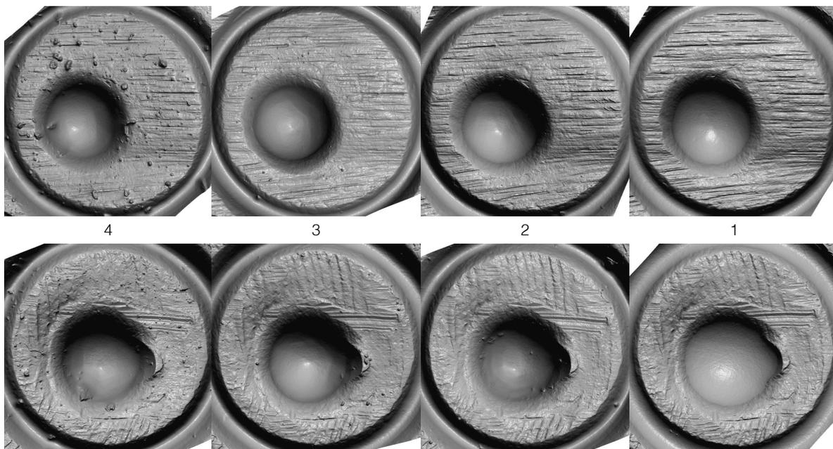
**Figure 3: Surface Contamination Score.** Each casing was assigned a value from 1-4 based on a human assessment of surface contamination (see text). (Top Row) Hi-Point 9mm; (Bottom Row) Norinco 9mm
