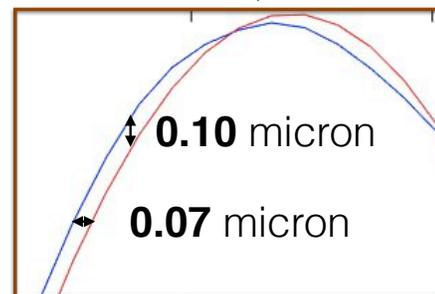
Figure 5: **Sinusoidal Reference Standard.** A system performance check was developed around a sinusoidal reference standard with wavelength 135 $\mu$ m and amplitude 19 $\mu$ m. An automated quality check analysis demonstrates that lateral and depth resolution is typically better than 1 $\mu$ m. See Section 3.
