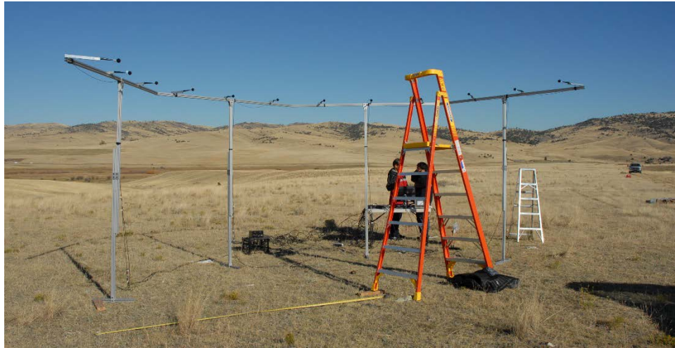
Figure 1: 3 meter radius x 3 meter tall aluminum custom-designed bracket with twelve instrumentation microphones attached for recording simultaneously at multiple azimuths.
