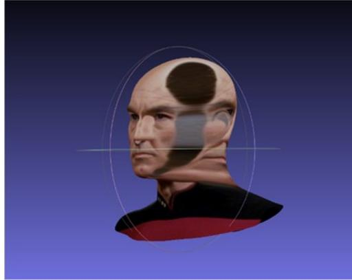
Figure 19: 3D Reconstruction showing self occlusion problem
