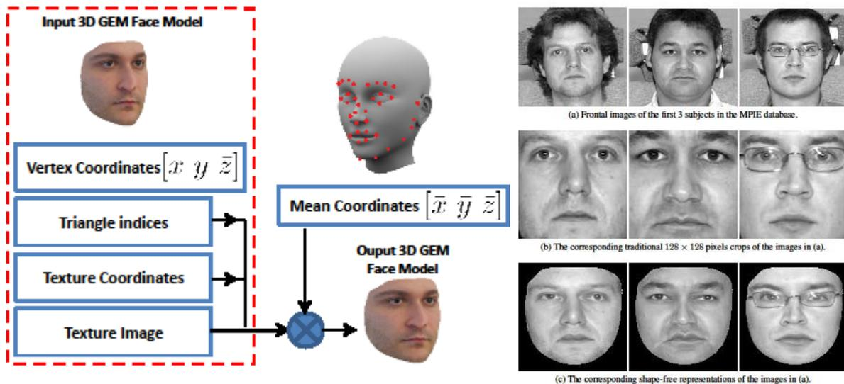
Figure 13: Generation of shape free images. The flowchart on the left depicts the procedure, while the images on the right depict example shape-free images (contrasted against traditional face crop)
