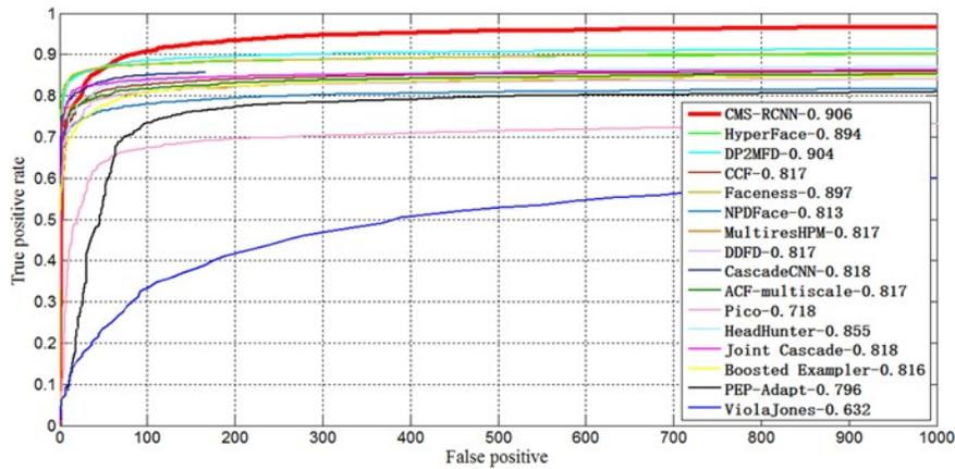
Figure 31: ROC curves of our proposed CMS-RCNN and the other published methods on FDDB database. Our method achieves the best recall rate on this database. Numbers in the legend show the average precision scores.
