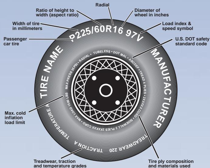
All tires contain very useful information molded into the sidewall. It shows the name of the tire, its size, whether it is tubeless or tube type, the maximum load and maximum inflation, the important safety warning, and much other information.
